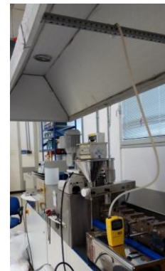
Figure 2. Extrusion line with ventilation on top
