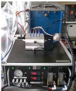
Figure 2. Experimental set-up: Test chamber in the rear, exposure unit and flow control in the front.
