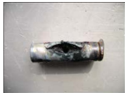
Figure 1. Destroyed cell after nail test. Electrical charge at test condition: 2.2Ah
