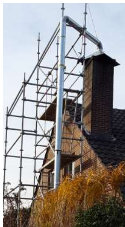
Figure 1: Sampling set-up for emission measurements of wood stoves under real life conditions.
