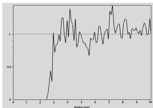
Figure 1. Pair radial distribution between molecules of water and ozone in the absence of Cr molecules
