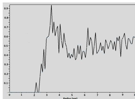
Figure 2. Pair radial distribution between molecules of water and ozone in aerosol cluster in presence of chromium molecules
