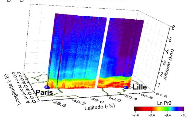
Figure 1. Lidar range corrected signal recorded during Lille-Paris mobile measurements
