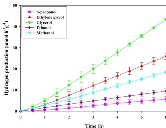
Figure 1. Comparison of the photocatalytic hydrogen production over Pt-GN/TiO<sub>2</sub> for different organic scavengers under UV-visible irradiation. Catalyst: 0.08 g; 10 vol.% aqueous solution (800 mL).
