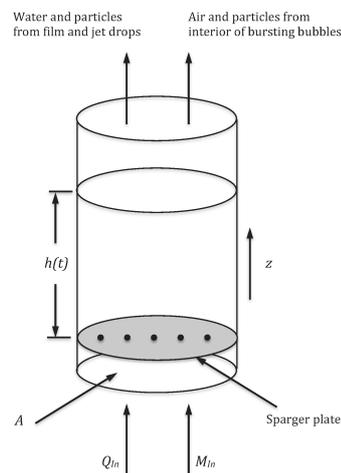
Figure 1. Bubble chamber used in experiments.  $A$  is the cross-sectional area of the bubble chamber,  $h(t)$  is the height of water in the chamber,  $z$  is the vertical dimension,  $Q_{In}$  is the flux of air in and  $M_{In}$  is the mass of particles in the air in.
