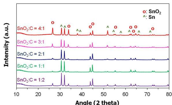
Figure 2. XRD diagram comparison of the carbon coated SnO<sub>2</sub> nanoparticles, under different SnO<sub>2</sub>:carbon black ratios.
