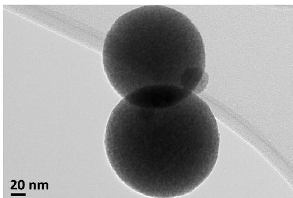
Figure 1. TEM image of SnO<sub>2</sub> nanoparticles synthesized by Aerosol Spray Pyrolysis
