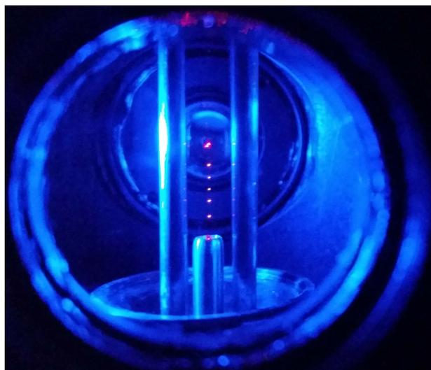
Figure 1. This is a photograph of 5  $\mu\text{m}$  polymer spheres confined in an LEQ. Two of the four vertical electrode rods are visible.
