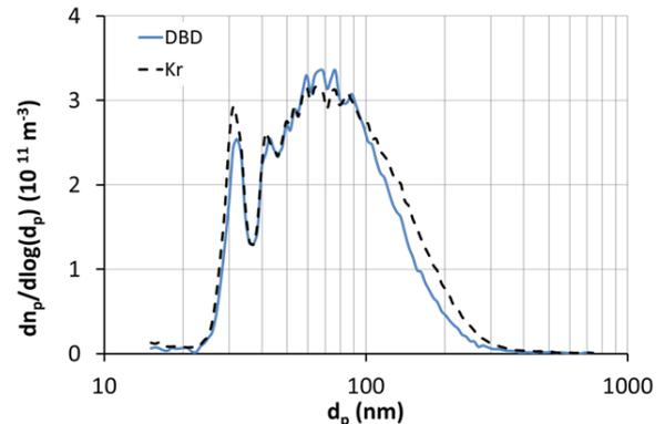
Figure 1. size distribution of poly-modal aerosol produced by nebulization of SiO<sub>x</sub> particle suspension  $d_p = 34$  nm &  $n_p = 2 \times 10^{11}$  m<sup>-3</sup> with air flow in the DBD.
