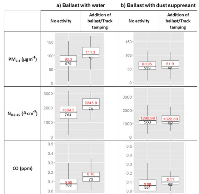
Figure 1. Box plot of PM<sub>2.5</sub>, N<sub>0.3-10</sub> and CO levels during subway operation hours, after ballast addition with and without dust suppressant. Data points in black, mean concentrations in red.
