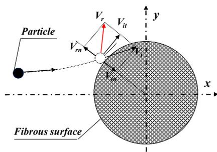
Figure 1. Schematic of particle impact and rebound on fibrous surface
