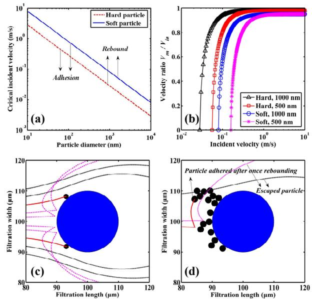
Figure 2. (a) The critical incident velocity as a function of particle diameter, (b) Velocity ratio ( $V_{rn}/V_{in}$ ) of soft or hard particles as a function of incident velocity, (c) Particle trajectory considering particle rebounding, (d) Particle deposition considering particle rebounding.
