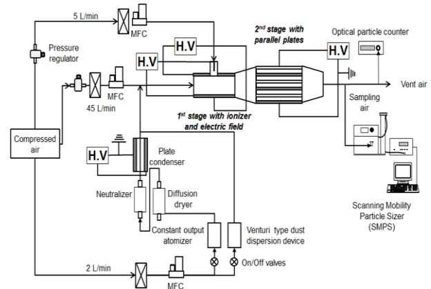
Figure 1. Experimental set up in this study.
