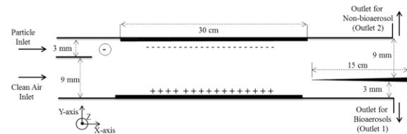
Figure 1. Schematic of the separator
