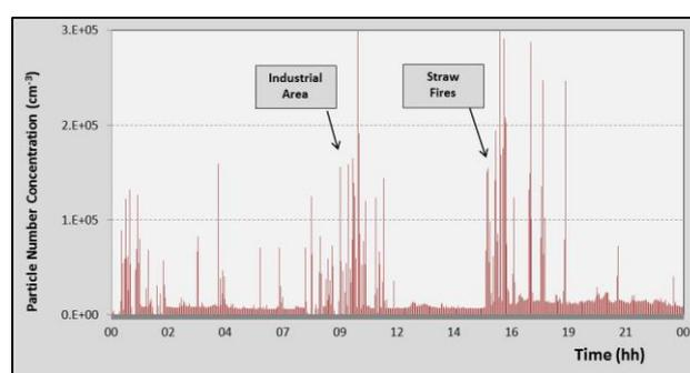
Fig 1: The PNC at 30s resolution obtained on the 27<sup>th</sup> of November. The spikes are due to combustion sources.
