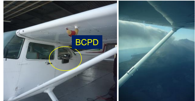
Figure 2 BCPD mounted on aircraft and view of the volcano plume prior to sampling.
