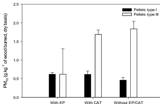
Figure 2. PM<sub>10</sub> emission factors for the combustion in a pellet stove with or without passage of the flue gas through a pollution control device.
