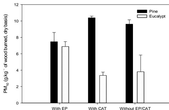
Figure 1. PM<sub>10</sub> emission factors for the combustion in the woodstove with or without passage of the flue gas through a pollution control device.
