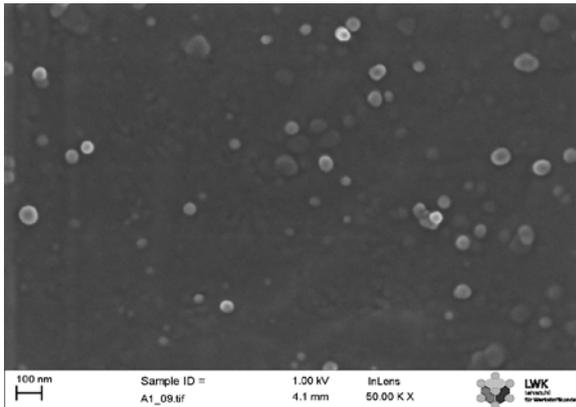
Figure 1. Exemplary SEM image of synthesized TiO<sub>2</sub> nanoparticles
