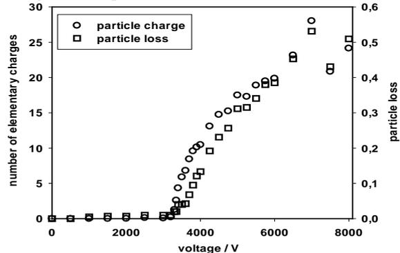
Figure 3. Number of charges per particle and particle loss for NaCl particles (100 nm mean diameter)
