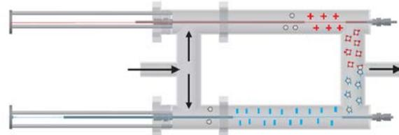
Figure 2. Designed parallel coaxial corona chargers.
