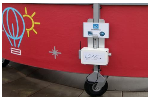
Figure 1 : LOAC on the gondola of the OAG balloon
