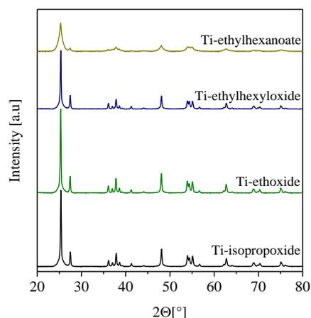
Figure 1. Diffragtograms of TiO<sub>2</sub> nanoparticles synthesized with different precursor salts in 2-methoxyethanol
