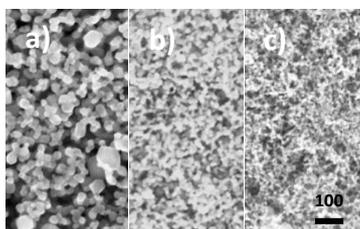
Figure 1. SEM images of pure a) ZnO, b) In<sub>15</sub>Zn<sub>85</sub>O, and c) In<sub>80</sub>Zn<sub>20</sub>O films (Kunzmann et al., 2015)
