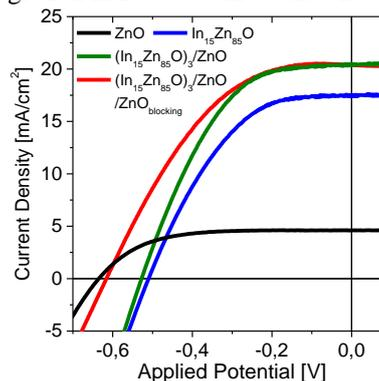
Figure 2. *J-V* curves of the devices featuring different photoanodes
